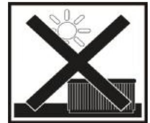
**Important note:** Do not leave your SPA uncovered in direct sunlight. The SPA has closed cell insulation foam under the shell. If left exposed to direct sunlight the surface temperature can build up to 200 °C causing damage to your SPA. It is suggested that you have the hard cover over your SPA while not in use. Leaving the SPA uncovered and exposed may void your warranty on your SPA and its accessories.
