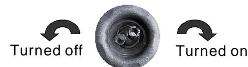
**Note:** Some jets and the air jets are unadjustable. Don't rotate these jets with force. It may cause damages to the jets.
